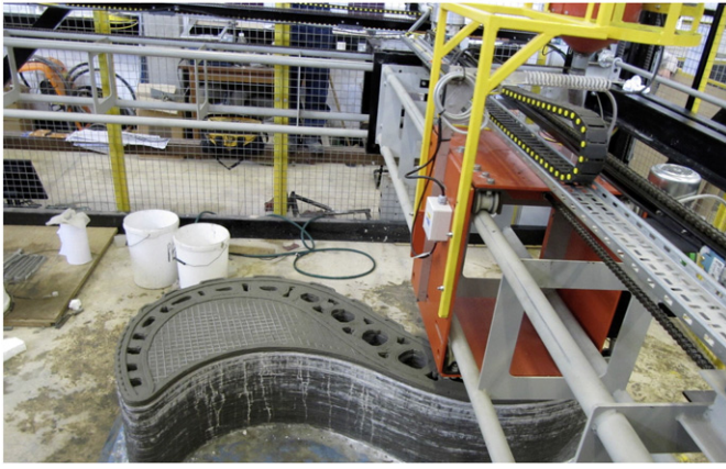
Fig. 4. 3D printing frame of Concrete Printing system [17].
