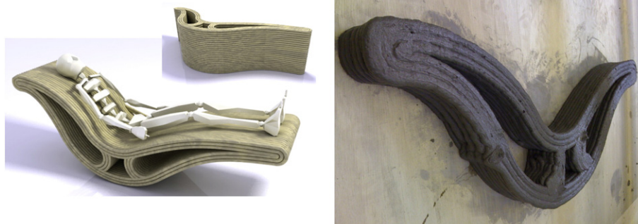
Fig. 8. Examples — bed. Left: CAD model and right: printed with a proprietary mortar product.
