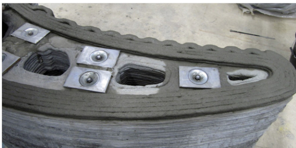
Fig. 10. Internal structure including functional voids and reinforcement.
